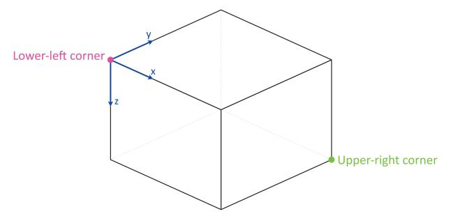
The final piece of information required to define the grid on which we will compute traveltimes is the node\_spacing between grid nodes along each axis (x, y and z). The LUT class will automatically find the number of nodes required to span the specified geographical region in each dimension. If the node spacing doesn't fit into the corresponding grid dimension an integer number of times, the location of the upper-right corner is shifted to accommodate an additional node.
